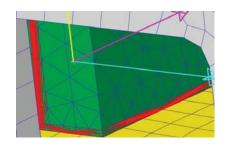
At this point, the machine was ready. We conduct a Static Analysis and a Frequency Response Analysis, comparing it to the sperimental tests we made at the factory. In Static Analysis we obtained errors of maximum **26µm** (other errors were **2**, **6** and **15** µm).
