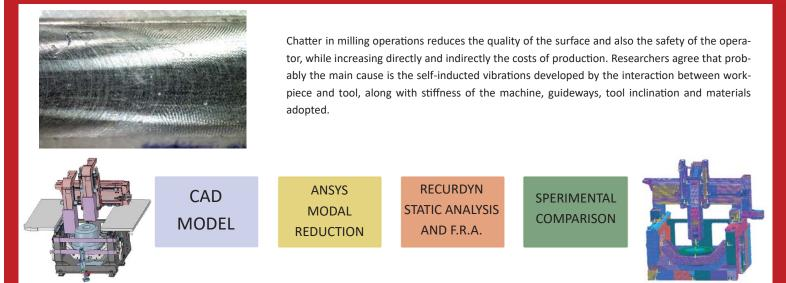
We reduced the whole 3D sketch of the CNC machine into an Ansys model. We discretised some parts as solids (e.g. guideways, tools, sliders) and some others as shells, allowing us to save a huge amount of nodes. We developed also a script in Ansys which allowed us to:
